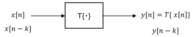
◆ The system is LINEAR if it obeys the principle of superposition:
